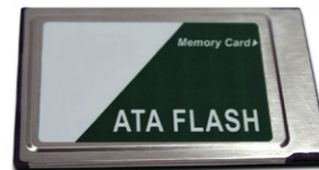
High-capacity PC card (PCMCIA) allows for storage of data from multiple aircraft flights
